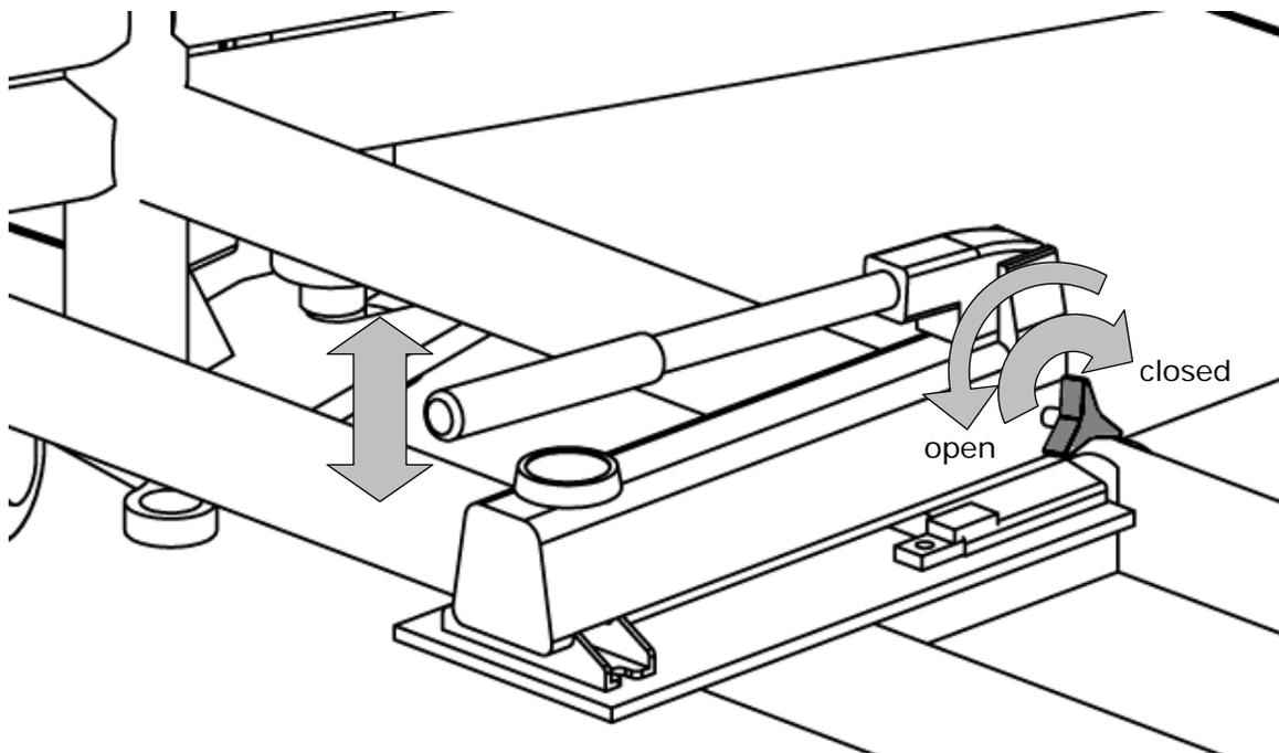
Make sure the vent knob on the hydraulic jack is closed. Use the jack to lift the tower far enough to allow easy movement. Do not move the tower alone; help is required to avoid objects on the floor and hanging objects. When the Tower is in place, open the knob slowly to drop Tower down to the floor. Move wings back to open position and replace lower panel.
