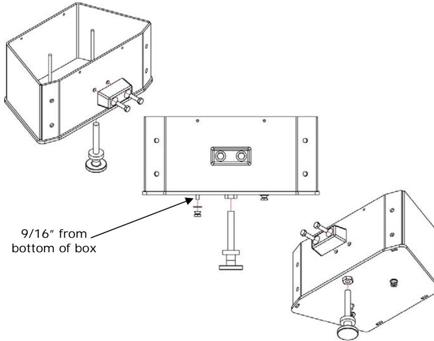
Assemble the counterweight box by installing screw foot, rubber bumper, and setting the threaded rods at the proper length. Approximately 9/16" of the rod should poke through the bottom of the box. Install tamper proof nuts and torque to break-off point, ~185-195 ft lbs.
