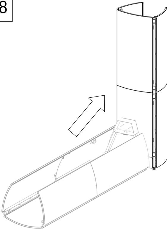
*Note: Use at least four people to raise any size tower! Place one person at the back of the tower to control counter-weight and prevent the screw feet from sliding. The other people are needed at the top of the tower to raise it by walking it up until all three screw feet are touching the floor.*
