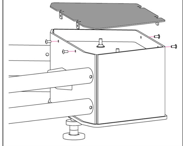
With the sound shell now upright, the counterweight plates can be installed. Test fit counterweight lid before torquing tamper proof nuts to breakaway at 185-195 ft-lbs. Finish by riveting lid closed.
