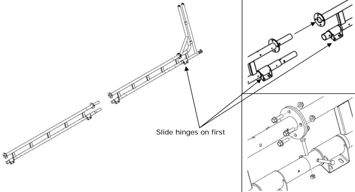
Make sure to add the proper hinge pieces before sliding the bottom and top mast tubes together. Bolt the connections as shown, with 3/8-16 x 2 1/2" bolts and nuts through the tube, and 3/8-16 x 1 1/4" flanged bolts and nuts through the plates. The L-shaped base and lower mast tubes connect in the same manner.
