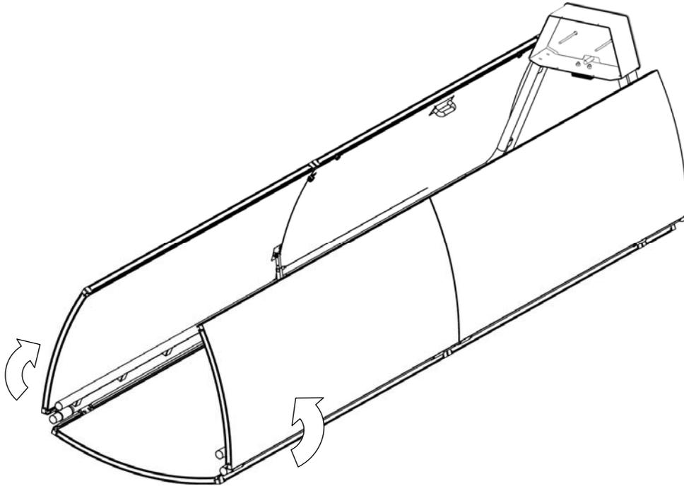
Pull the ropes on the hinge stop bracket and raise both sides of tower to a vertical position until they lock into place.
