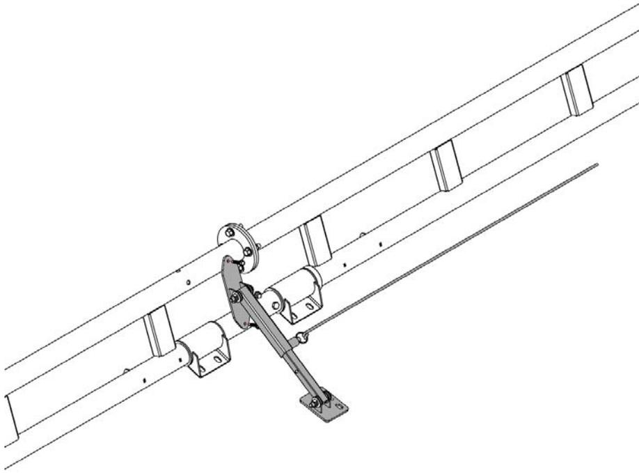
Use  $\frac{1}{4}$  x  $1 \frac{1}{4}$ " Tec screws to fasten sound shell wing arms to the mast tubes.
