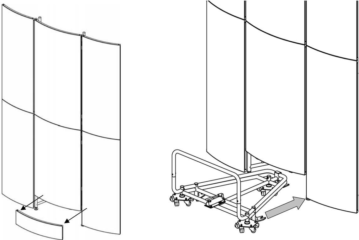
Remove lower panel of the tower, and roll tower mover into place. Make sure the floor is clear of debris and there are no obstructions hanging from the ceiling.
