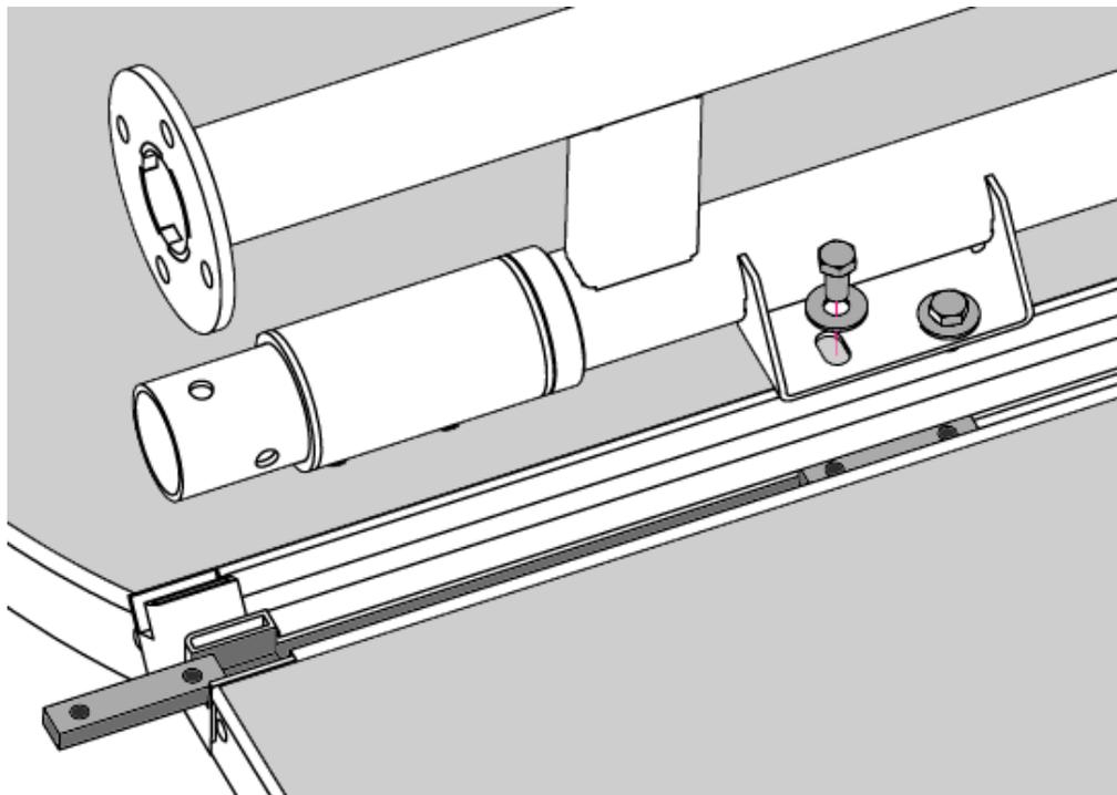
Attach masts to back side of panels by sliding strut nuts, one for each hinge bracket, into the track slot. Line up each strut nut with its corresponding hinge bracket and fasten with  $\frac{3}{8}$ -16 x  $\frac{3}{4}$ " bolts and washers.
