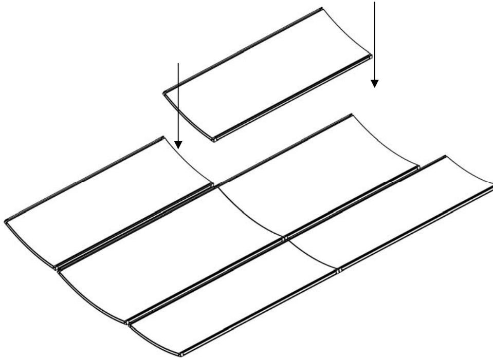
Lay the panels out face down on the floor according to the map. *Note: Make sure the floor is clean to help prevent damage to the panels.*
