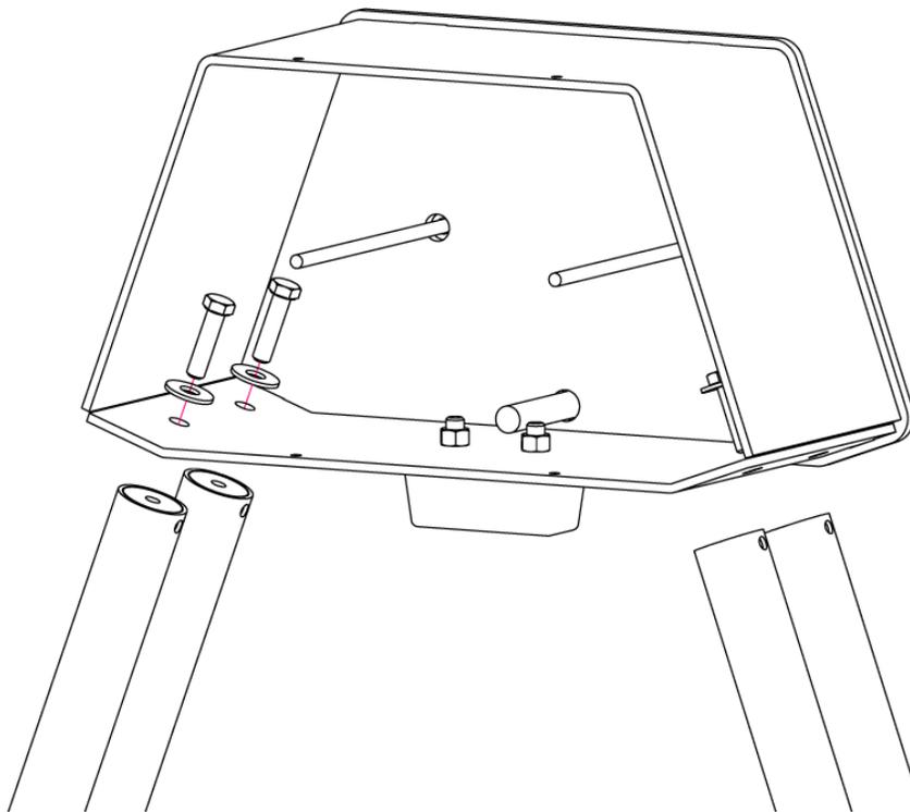
Install the counterweight box with four 1/2-13 x 2" bolts, washers and nuts.
