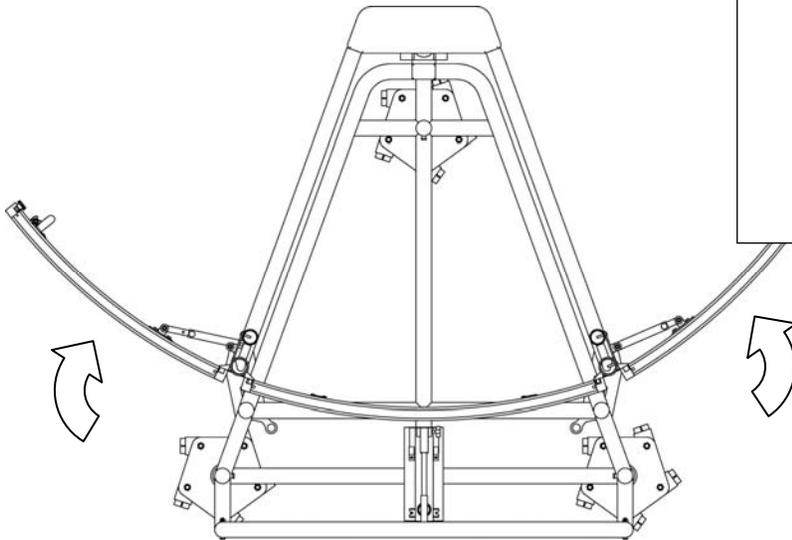
Move tower wings into the mid-span position, and roll the mover into place. Lift plates must be fully engaged on lift puck before lifting.
