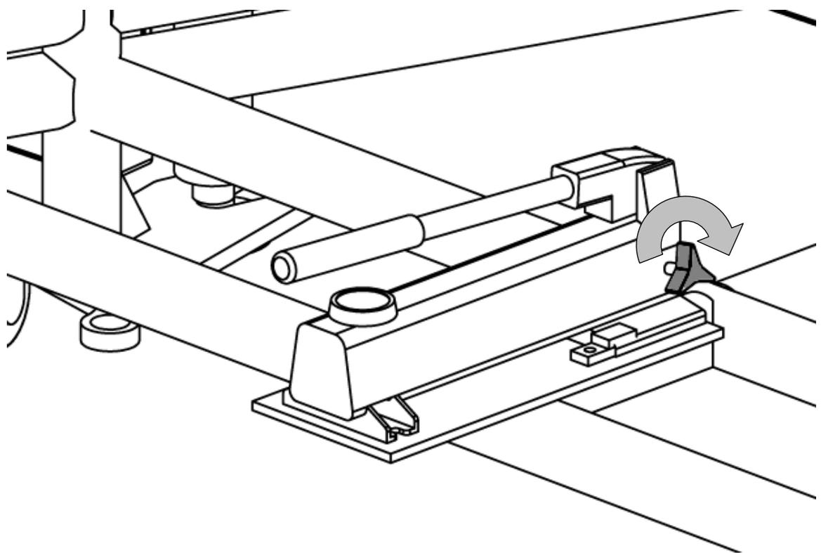
Tighten knob to avoid loss of pressure.
