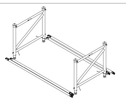
Begin the assembly of your ME - 1000AT Support System by laying out the components as shown above. Take note that the horizontal braces are marked with a green sticker while the diagonal braces are marked with a yellow sticker. Assembly of this structure should be done with at least two people and tools are not required.
