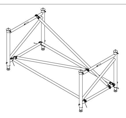
Complete the assembly by attaching the final diagonal brace.
