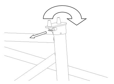
To change the position of the locator nodes begin by pulling the spring pin that keeps the locator assembly in place and rotate the locator to the desired position and then release the spring pin.
