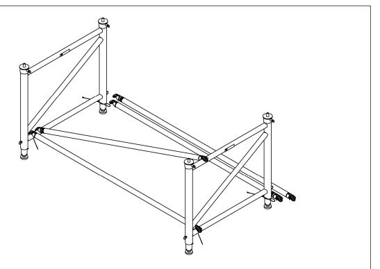
Next attach one of the diagonal braces to the assembly as shown above. Simply attach one end of the brace to the lower level of the H-section and then attach the opposite end to the top level of the H-section.
