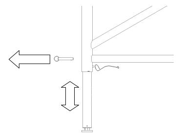
To select stage heights in two inch increments, simply remove the faspins from the leg tubes and then raise or lower the tubes to the desired height. Once the desired height is obtained, re-insert the faspins. If using an even number of decks, two understructures must be next to each other.
