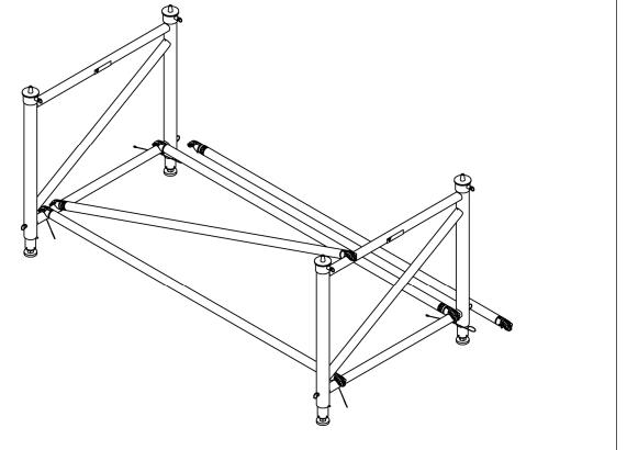
Attach the remaining horizontal brace as before.
