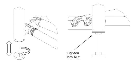
To level the deck after it has been placed on the ME-1000 Support System, simply raise or lower the adjustable screw feet by threading them in or out. Once the deck has been leveled, go back and tighten down all of the jam nuts on the screw feet to hold that position.
