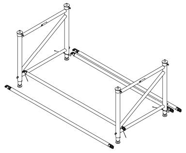
Start by assembling one of the horizontal braces as shown above. Attach one end of the horizontal brace to an H-section and then move the opposite section accordingly so that it can be hooked by the other end of the brace. It is recommended that you attach the horizontal braces as close as possible to the vertical tube of the H-section.
