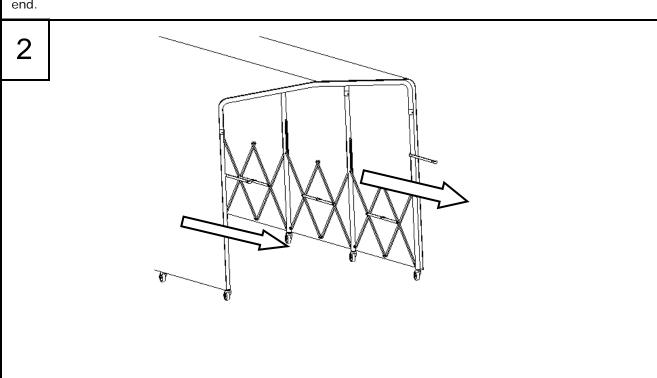
Pull the collapsed Player Tunnel into extended position.
