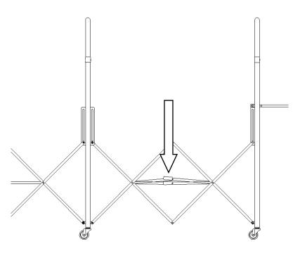
Push lock handle to over-center position to initiate lock between all vertical posts. Place outer covering onto frame and attach with Velcro straps. Make sure all straps are secured properly.
