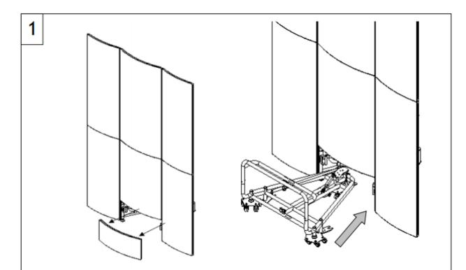
Remove lower panel of the tower, and roll tower mover in front of the tower as depicted above. Make sure the floor is clear of debris and there are no obstructions hanging from the ceiling.
