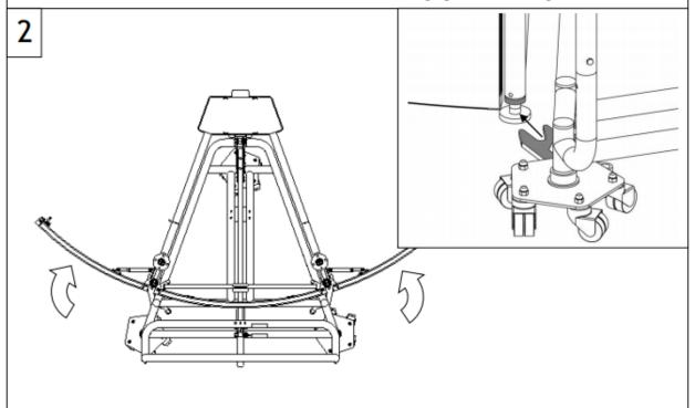
Verify that the mechanical lifter handle is locked in the upright position. Move tower wings into the midspan position, and roll the mover into place. Lift plates must be fully engaged on lift puck before lifting.
