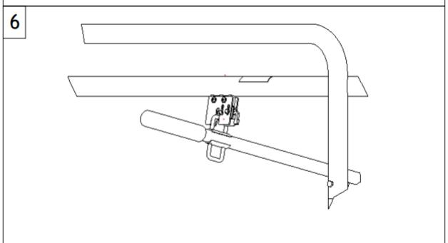
Lift the mechanical lifter handle until the it is locked securely into the top lock mechanism. Pull mover out from underneath the tower. Move wings back to open position and replace Lower panel.
