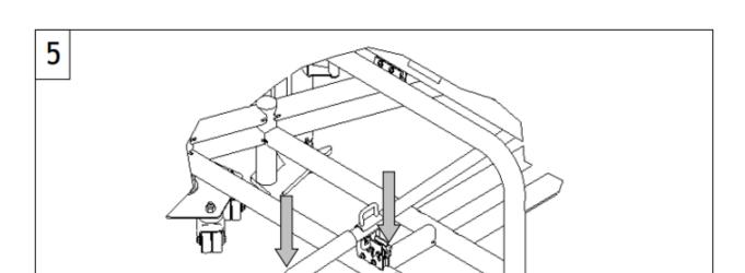
When the Tower is in place, press downwards on the mechanical lifter handle while simultaneously releasing the lock with the other hand. Maintain resistance on the handle until to sound shell rests safely on the floor.
